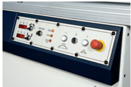
S40M control panel with switches for saw unit lifting and tilting and electronic digital readouts
