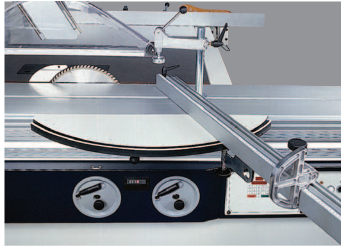
Angular cutting device with automatic stop position compensation relative to the blade. Each time the cutting angle is adjusted so that the distance between the stop and the blade remains constant. This enables rapid set-up and reduces test cutting.
